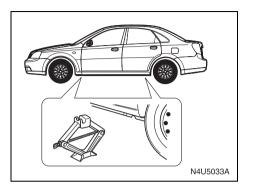
Near each wheel well is a notch in the frame which the jack head fits in.
